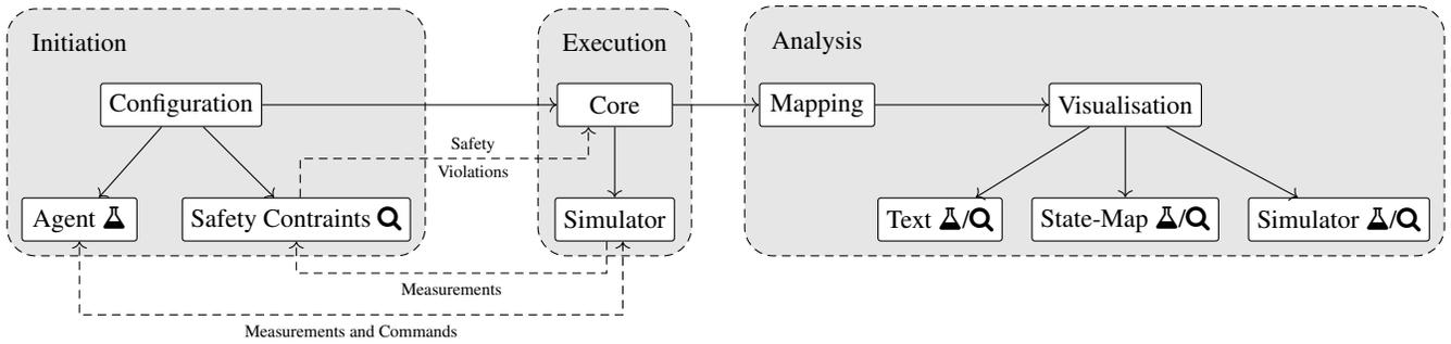
Figure 1: Architecture of the framework — Roles: Developer  $\Delta$ , Safety-Engineer  $\mathcal{Q}$
