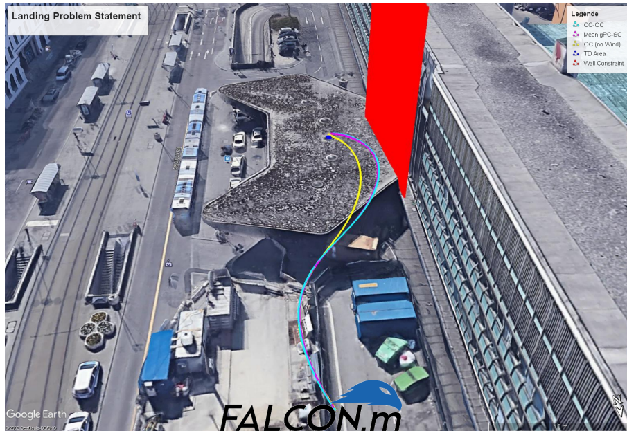
Figure 9.24: Visualization of landing setup including constraints (blue touchdown cylinder; red area for building), optimal results with no wind (yellow), mean generalized polynomial chaos stochastic collocation solution (magenta), and chance-constrained optimal control solution (cyan).
