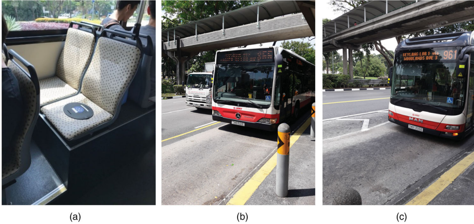
Figure 3. Field measurement setup. (a) On-cushion Svantek SV100A. (b) The Citaro single-decker bus. (c) The MAN NL323F.
