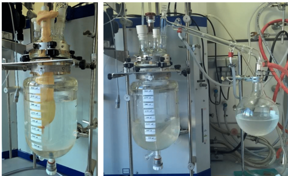
Supplementary Figure 3: Enzyme bag loaded with Novozyme-435 for epoxidation of (+)-3-carene ( 1 ) to epoxide 2-35 (left) and azeotropic distillation of cyclohexane before the Meinwald rearrangement of epoxide 2-35 to ketone 3-35 catalysed by \text{Fe}(\text{ClO}_4)_2 \cdot \text{H}_2\text{O} (right) in the 4.0 L scale.
