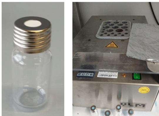
Supplementary Figure 17: Pictures of the reaction vial and oven for polymerization method B.
