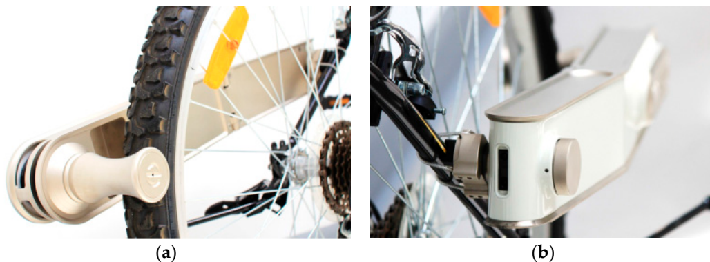
Figure 4. (a) Friction roller engagement; and (b) mounting and proximity sensor.
