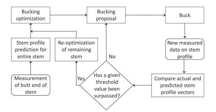
**Fig. 3.** Flowchart indicating the general steps of the bucking optimization proposal (Uusitalo 2010).
