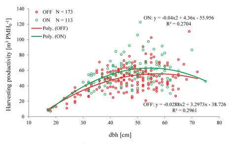
**Fig. 6.** Harvesting productivity  $[m^3 PMH_0^{-1}]$  in function of tree dbh for all harvested trees with pre-harvest inventory data.
