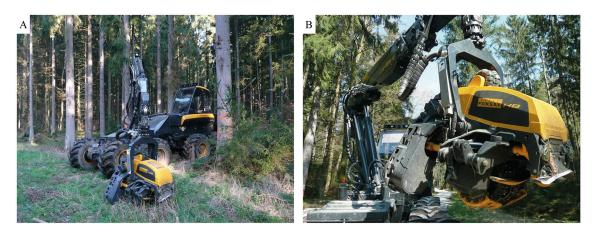
Fig. 2. A. Ponsse Bear single grip-harvester, B. Ponsse H8 harvesting head.
