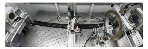
Fig. 10. Wide-angle view of the actual setup. From left to right: X-ray source (T) with source grating ( $G_0$ ) directly in front of it, at the center the phase grating ( $G_1$ ), then the Euler cradle with sample (S), and adjacent to it the analyser grating ( $G_2$ , in the cross-shaped holder); behind the latter the X-ray detector (D, hidden).
