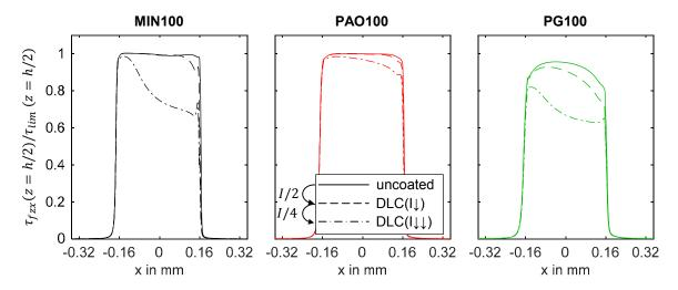
**Figure 5.** Shear stress  $\tau_{fzx}$  related to the limiting shear stress  $\tau_{lim}$  for MIN100, PAO100 and PG100 and for uncoated and coated gears for the highest local gear power loss  $P_{VZP}(\overline{y})$  along the path of contact.
