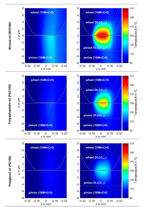
**Figure 4.** Temperature distribution for uncoated (**left**) and DLC( $I\downarrow\downarrow$ ) coated (**right**) gears for MIN100, PAO100 and PG100 for the highest local gear power loss  $P_{VZP}(\overline{y})$  along the path of contact (close to B).
