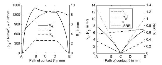
**Figure 2.** Line load w, Hertzian pressure  $p_H$  and radius of curvature  $R_x$  (**left**) and sum velocity  $v_{\Sigma}$ , sliding velocity  $v_g$ , slip ratio s and slide-to-roll ratio SRR (**right**) along the path of contact of the considered FZG type Cmod gear.
