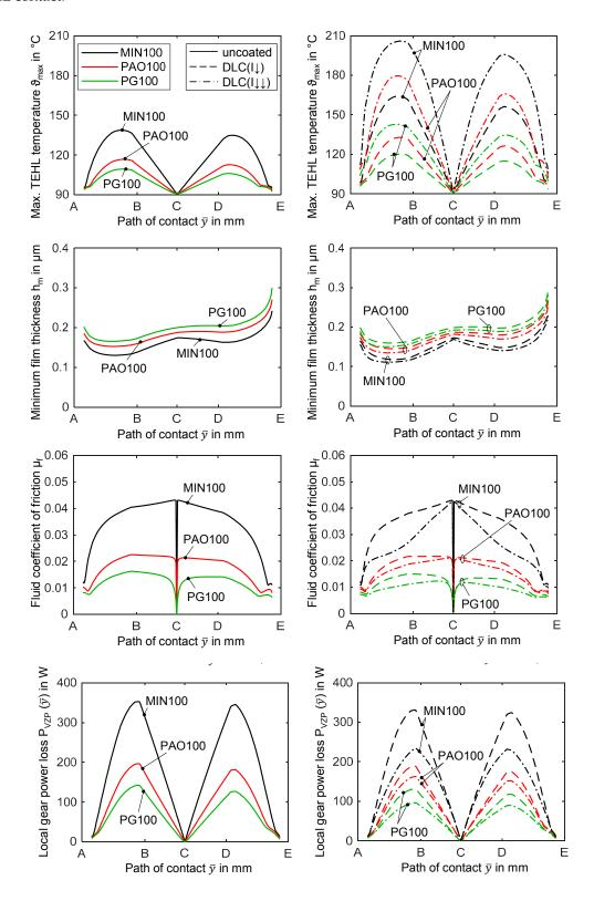
**Figure 3.** Maximum TEHL temperature  $\vartheta_{max}$ , minimum film thickness  $h_m$ , fluid coefficient of friction  $\mu_f$  and local gear power loss  $P_{VZP}(\overline{y})$  for MIN100, PAO100 and PG100 along the path of contact for uncoated (**left**) and coated gears (**right**).
