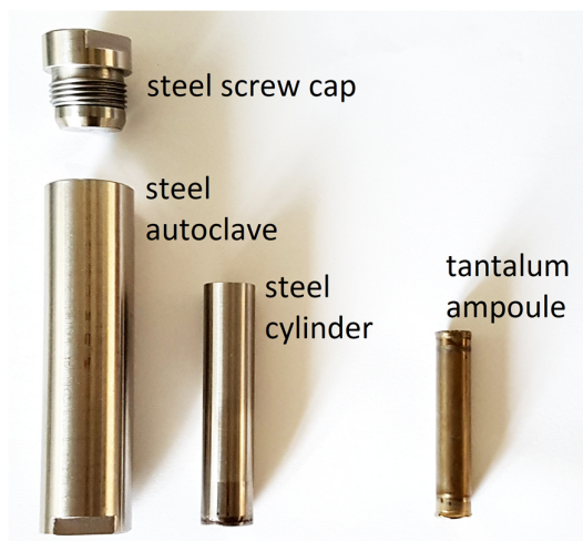
Figure 34. Stainless-steel autoclave (for K_4Ge_9 ) and tantalum ampoule (for K_4Si_4 and K_{12}Si_{17} ) as used for the solid-state syntheses of Zintl precursor phases.
