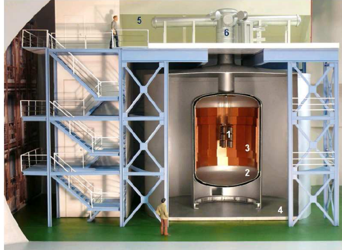
Figure 2.3: Artistic view of the GERDA experiment. The germanium detector array (not to scale) (1), inside the LAr steel cryostat (2) with its internal copper shield (3) and the surrounding water tank (4). The clean room is located above the water tank (5) around the cryostat neck (6).
