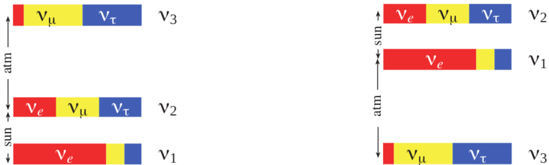
Figure 1.1: Summary of the neutrino parameters derived from oscillation experiments. The scenario on the left is for the normal ordering and the inverted ordering is shown on the right side. The colours represent the flavour composition of the three mass eigenstates. Figure from [35].
