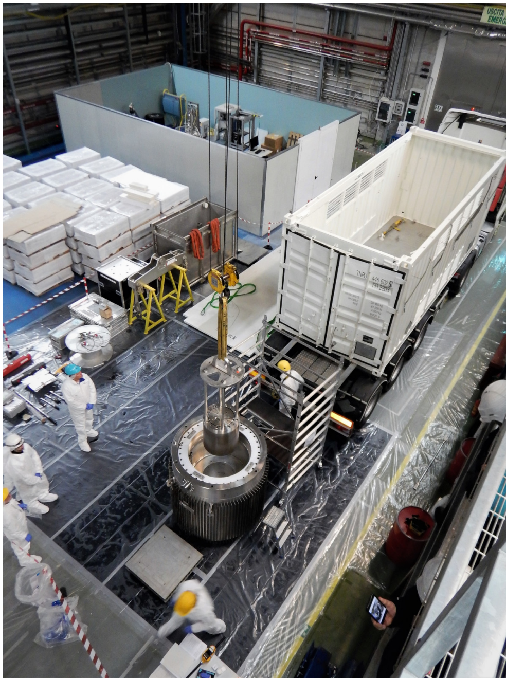
Figure 5.17: The extraction of the tungsten shield from the casket to demonstrate the safe handling of a radioactive source during the ISPRA test. The floor is covered with plastic to contain possible radioactive contaminations. During these tests no actual radioactive material was used, in contrary to local news reports.
