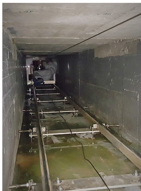
Figure 2.5: The insertion of a source mockup into a calorimeter in the clean room (left) and the pit with the rail system (right).
