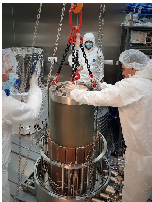
Figure 2.5: The insertion of a source mockup into a calorimeter in the clean room (left) and the pit with the rail system (right).
