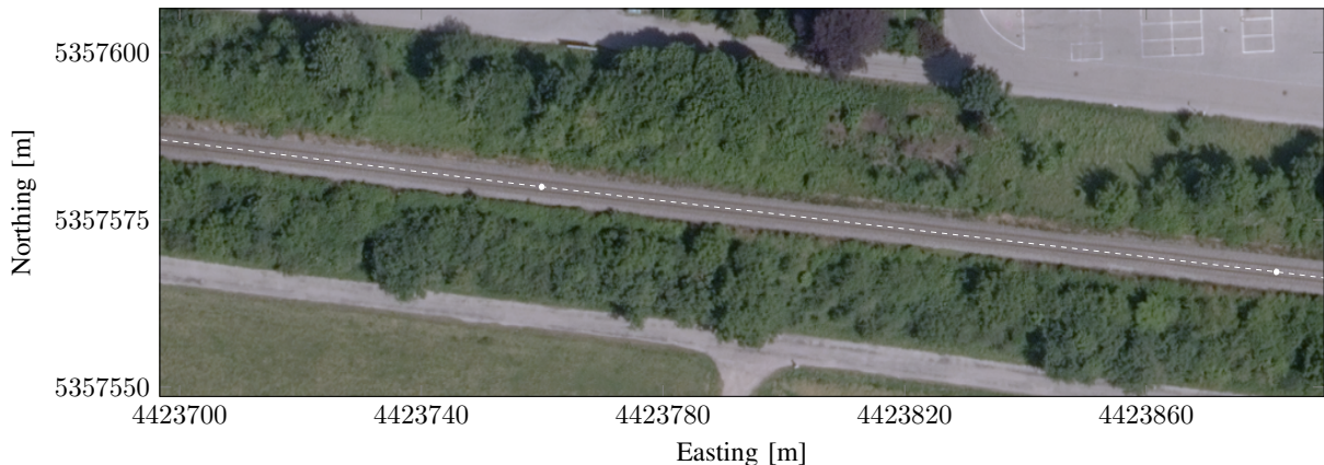
Figure 7.7: Geo-referenced digital orthophoto with a sampled track (white) of the reference track map.
