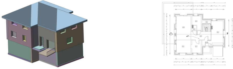
Figure 5: Visualization of a BIM model as a standard 3-story residential building, and its corresponding floor plan portraying the ground floor derived at 1.20m level.
