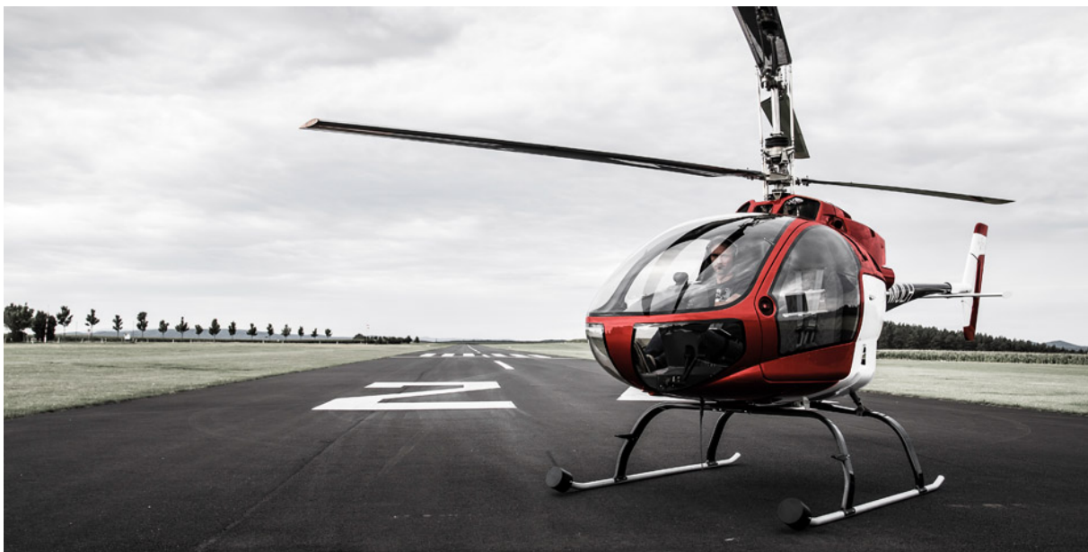
Figure 1.4: Photographic Image of the Technology Demonstrator: The Coaxial Ultralight Helicopter by edm aerotec GmbH (CoAX 2D) [55]
