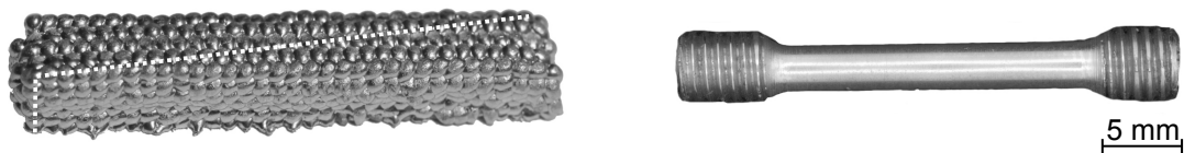
Figure 4.10: Printed block of AlSi12 (left) and tensile specimen (right). A white dotted line shows the cutting plane for the micrographs.
