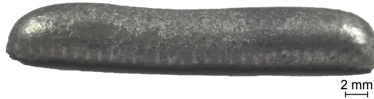
Figure 5.28: Images of an Al99.5Ti specimen printed at T_{\text{subs}} = 654 °C. Sharp corners and the overall shape are lost.
