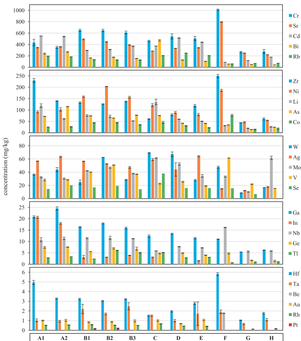
Fig. 3. Concentrations of trace components (triplicate average, single measurement in the case of Se) except rare earth elements in the fly ash samples A–H. Concentrations that are below the LOQ are not shown in the diagram. The error bars represent the standard deviation of the triplicates.
