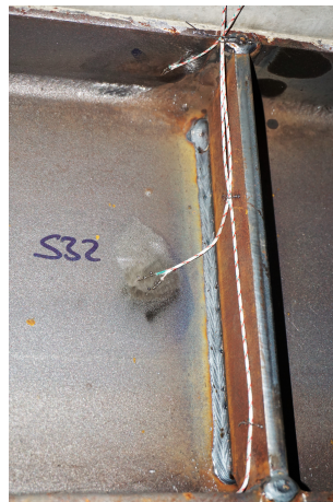
Figure 3.7: Welded thermocouples on the steel section
