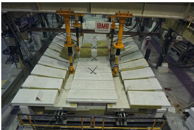
Figure 3.14: Left: Picture of the test set-up during the fire experiment Right: Cross section of the test set-up, from [33]
