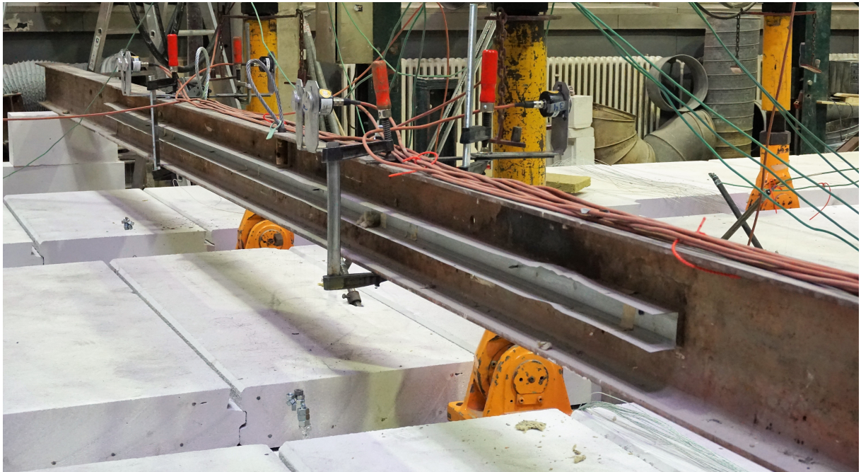
Figure 3.10: Reference beam for measuring the vertical deflection
