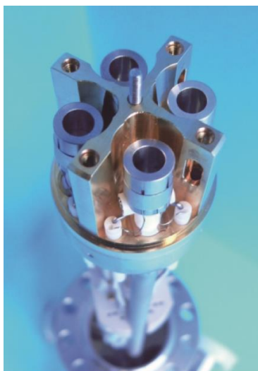
Figure 2.10: Image of OMBE with 4 independent crucibles, from Dodecon Nanotechnology GmbH .
