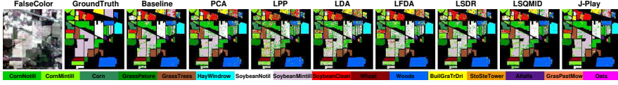
Fig. 3. A false color image, ground truth and classification maps of the different algorithms obtained using CCF on the Indian Pines dataset.
