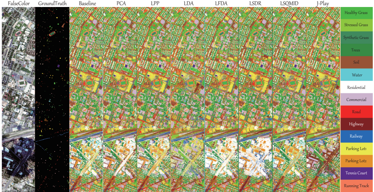
Fig. 4.9. A false-color image, groundtruth, and classification maps of the different algorithms obtained using CCF classifier on the Houston2013 dataset with the corresponding categories.
