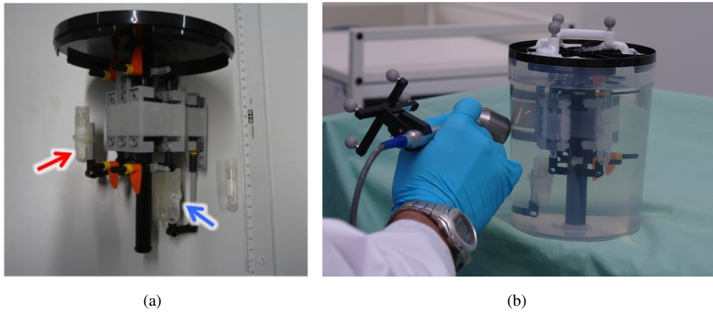
Figure 5.2.: Phantom construction. (a) The neck phantom was constructed by using a plastic cylinder (very close to the human neck in dimension) and three 2 ml laboratory reservoirs: two were rigidly glued to each other for simulating the tumor (blue arrow), and a third one was used for simulating the lymph node (red arrow). (b) A tracking target was attached on top of the phantom, and after preparation with ^{18}\text{F} -FDG, the phantom was scanned using our system.
