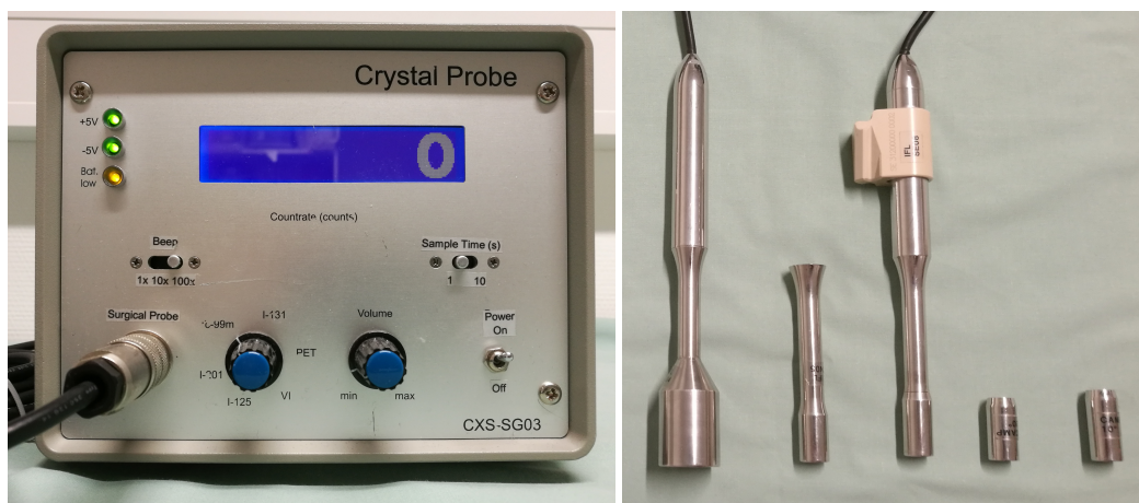
Figure 3.3.: Crystal Probe gamma radiation detection system in declipseSPECT. Left: Controlling unit SG03. Right: High-energy and standard straight gamma detection probes with interchangeable collimators.
