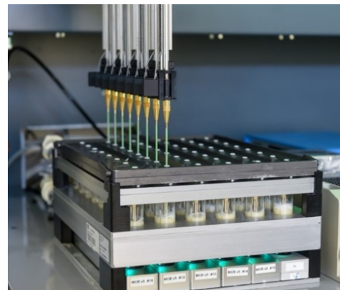
(b) Bioreactor block and active pipetting arm of the liquid handling system (Image copyright: Institute of Biochemical Engineering, Technical University of Munich)
