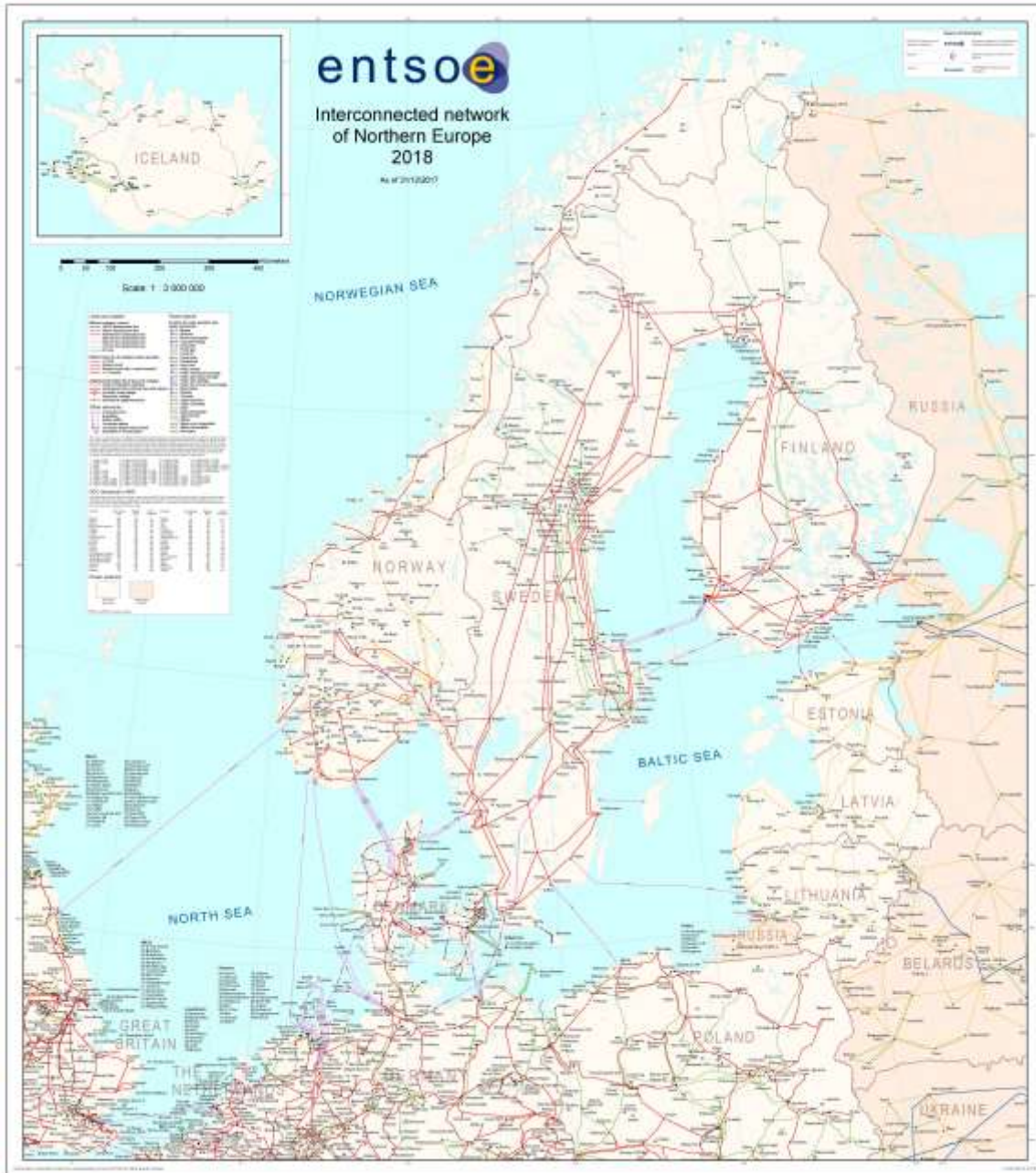
Figure 9: Illustration of the transmission system network operated by members of the European Network of Transmission System Operators (TSOs). Network elements are located only at their approximate geographic location. Important transmission sections, generators and substations in the so called Nordel area and neighboring areas are shown; use permitted by Entsoe (2018) 3 .
