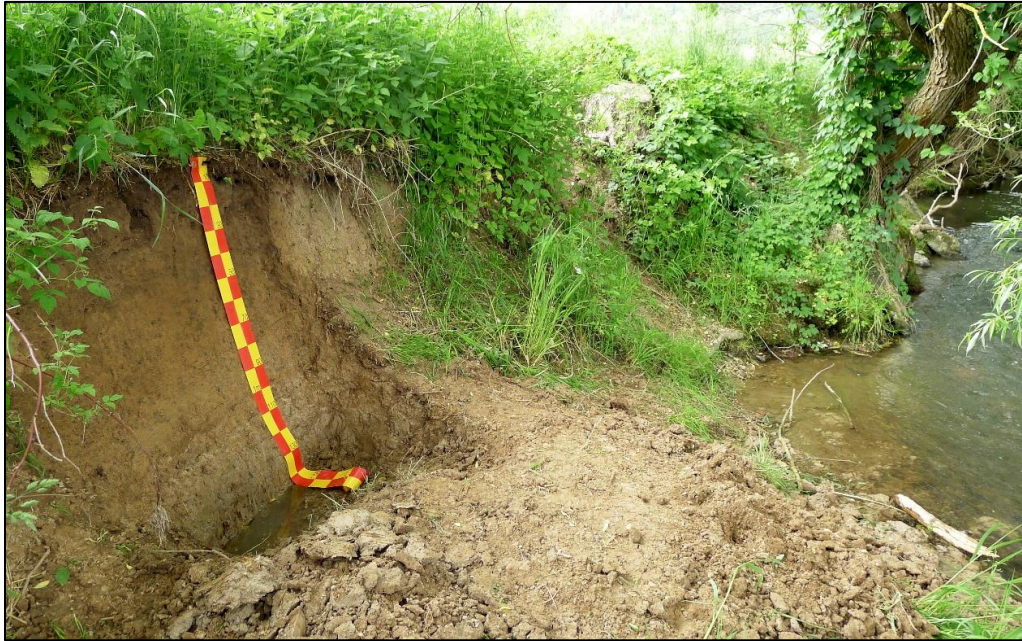
Figure 3: Soil profile at the eroded bank crest of the Otterbach River (profile data not shown) (Foto: S. Kriegs, 2015).
