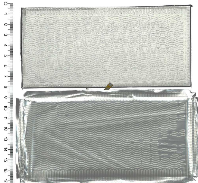
(c) Dismantled bottom cover showing the resistive sensor mesh (scale as reference in cm). Its connector only carries the three signals MeshGND, MeshSigIn, and MeshSigOut.
