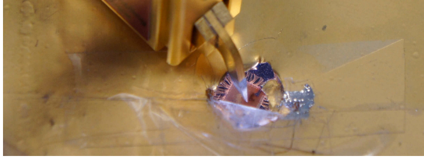
(a) Photo of the advanced attack with field probe above decapsulated IC.
