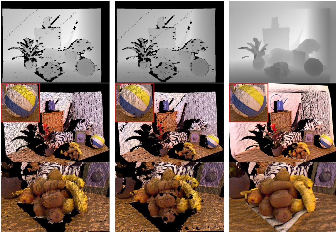
Figure 4.6: Depth maps (top row), 3D rendering of Kinect color and depth data depicting the entire scene (middle row) and a detail of the fruit bowl (bottom row). Left column: original Kinect data like in the top row of Figure 4.5 with downsampled color information, center column: bicubic interpolation (1280x960), right column: proposed method (1280x960). Note that object shadows are due to the single view occlusions.
