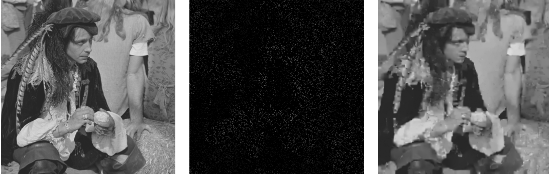
Figure 3.6: Original version (left), 5% of its pixels (middle) that are used as the input to the algorithm and the reconstructed version (right) of the test image 'man'.
