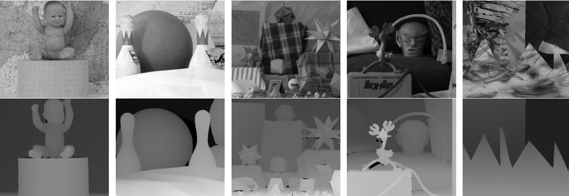
Figure 4.4: The five training images from [154] used for learning the bimodal intensity-depth analysis operator. The intensity images (top) and corresponding depth maps (bottom) are spatially registered prior to sampling patch pairs for training.
