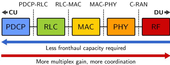
Fig. 1. Possible functional splits for the 5G RAN, where each function is a layer of the protocol stack (incomplete list). The functions to the left of each split are located in the CU, whereas those to the right are in the DU.
