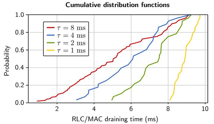
Fig. 5. Cumulative distribution functions of the RLC/MAC draining times for different inter-arrival times  $\tau$ . Each curve corresponds to 100 migrations.
