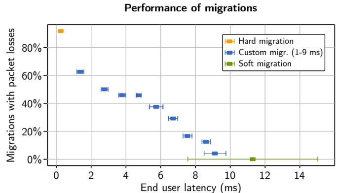
Fig. 6. Number of migrations experiencing one or more packet losses as a function of the maximum end-user latency. Nine custom migrations are shown, with allocated times ranging from 1 to 9 ms. Each point represents 20 migrations from MAC-PHY to PDCP-RLC.
