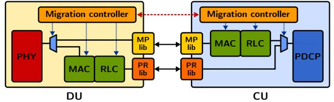
Fig. 3. Functional architecture of the two binaries supporting an adaptive functional split. The blue trapezoid symbolizes the ability of the migration controller to steer the flow of data.
