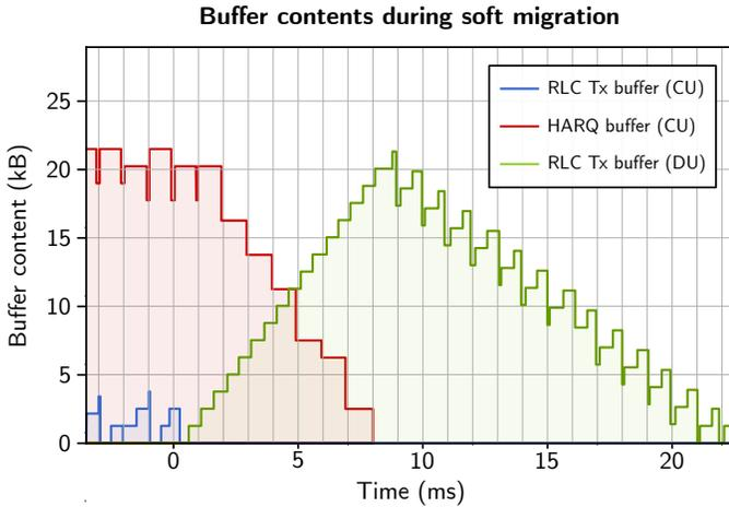
Fig. 4. Content of the RLC and HARQ buffers during a soft migration. The input traffic is a constant-rate 20 Mb/s stream, and the network downlink capacity is 31.7 Mb/s. The migration starts at  $t = 0$  ms.
