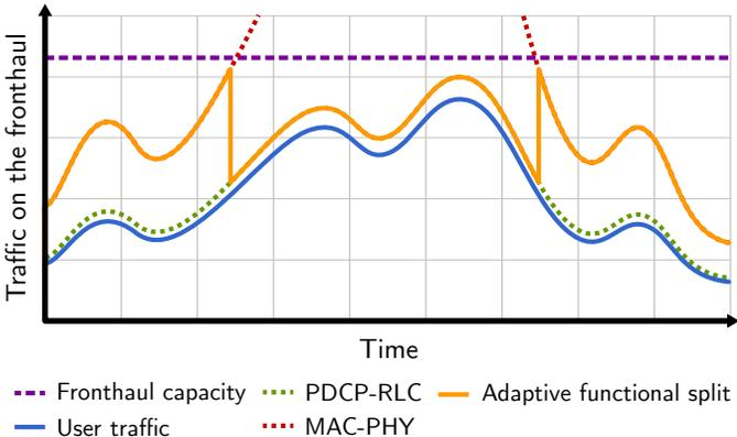
Fig. 2. Example of the fronthaul traffic produced by a 5G RAN implementing a PDCP-RLC split, a MAC-PHY split, and an adaptive functional split as a function of the user traffic.
