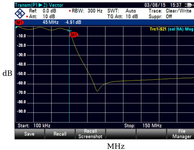
Figure 6.6.: Measured frequency response of the low-pass filter
