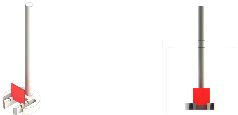
Figure 3.1: 3D drawing of the PTFE sample holder used for handling the silicon sample (red) inside the beaker during the cleaning and etching steps.
