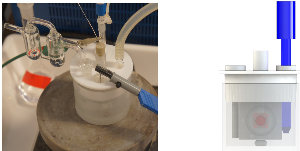
Figure 3.4: Picture (left) and 3D drawing (right) of the electrochemical cell. The three electrodes depicted in the rendering are colorcoded as follows: RE (blue), silicon WE (red) and glassy carbon CE (gray). Picture from the master thesis of Andreas Heine [27].
