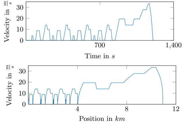
Figure 1: Top:  $v_{x,tar}(t)$ -curve, bottom:  $v_{x,tar}(x(t))$ -curve of the NEDC
