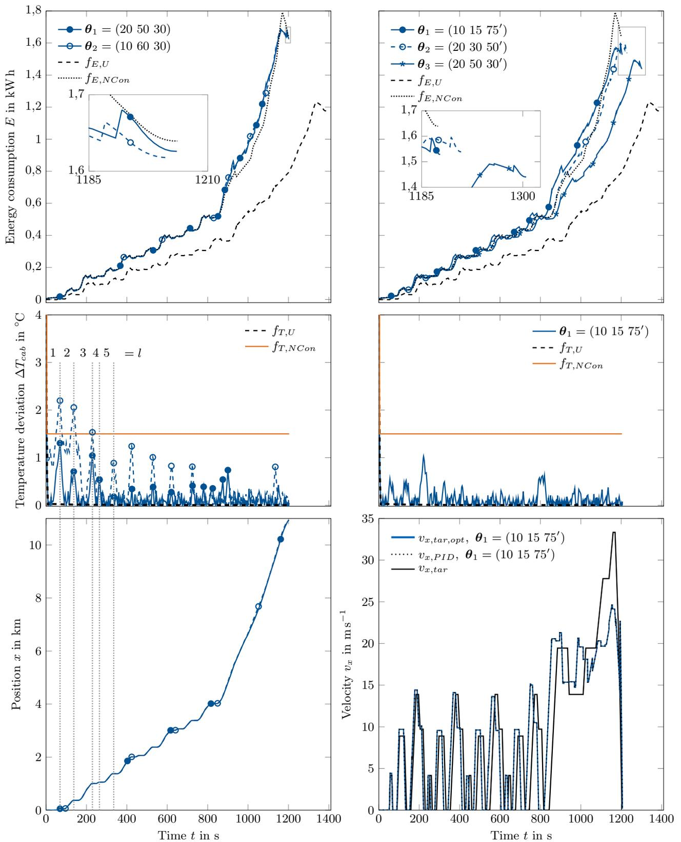
Figure 2: Sliding window approach with same decision maker priority vectors  $\theta_{1/2}$  as in the optimization of an entire driving cycle (left); sliding window approach with the decision maker priority vectors  $\theta_{1/2/3}$  using  $f'_t$  instead of  $f_t$  (right)
