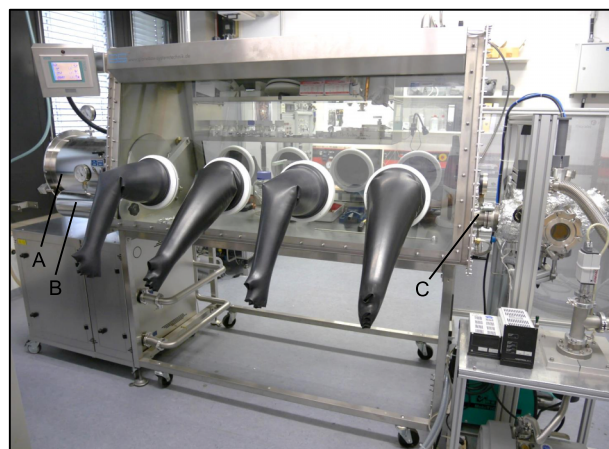
FIG. 1. Commercial argon glovebox from GS as equipped with various bespoke components. The glovebox includes three locks (A), (B), and (C). On the right-hand side, the arc melting furnace is connected to the glovebox via lock (C).
