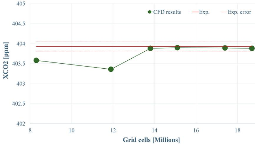
(b) Comparison XCO<sub>2</sub> using 6 different mesh sizes
