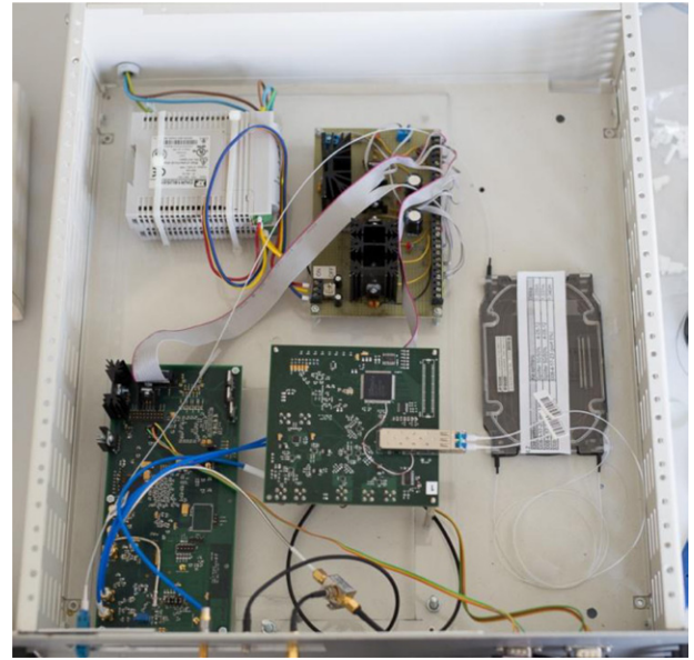
Figure 4. The inside of the TWOTT terminal. In front, from left to right, there are the event timer, the TWTT board, and optical splitters.
