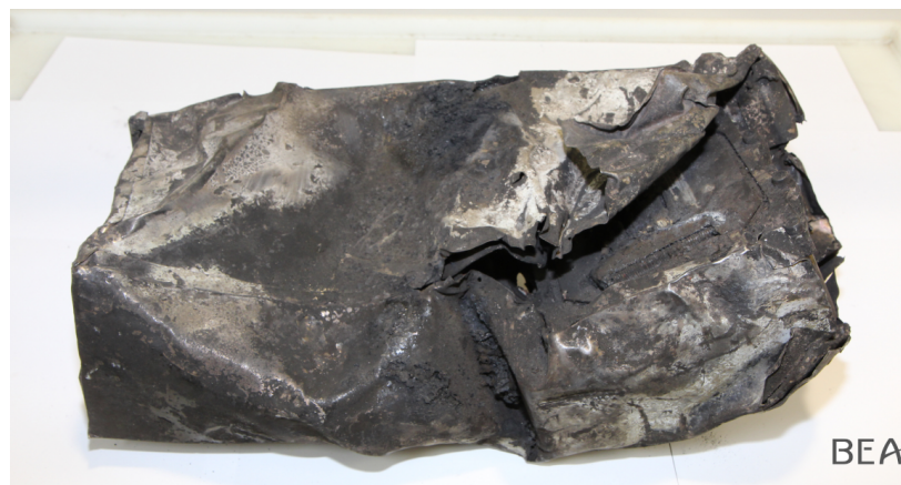
Figure 2.4: The heavily damaged, but still readable FDR of the A320 that crashed in the French Alps after recovery [Bur16]
