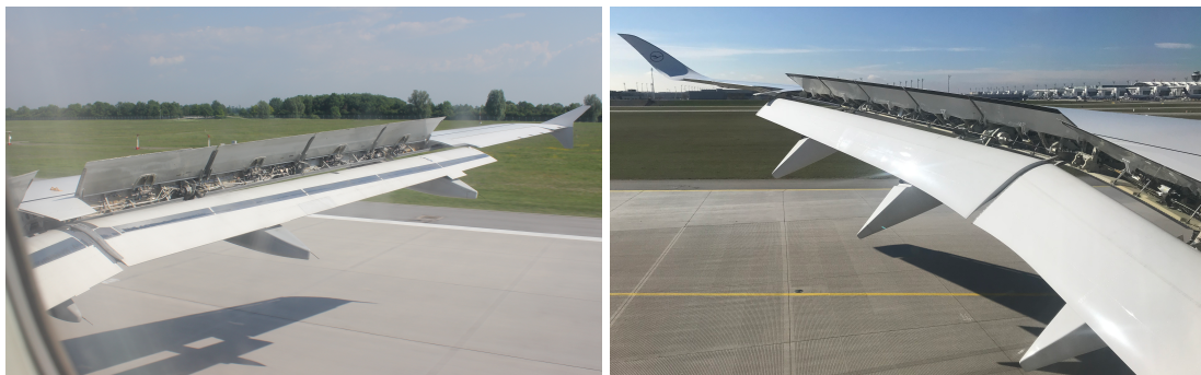
(a) Spoiler deployment on the Airbus A320 (b) Spoiler deployment on the Airbus A350 with no use of the aileron with ailerons deflected upwards
