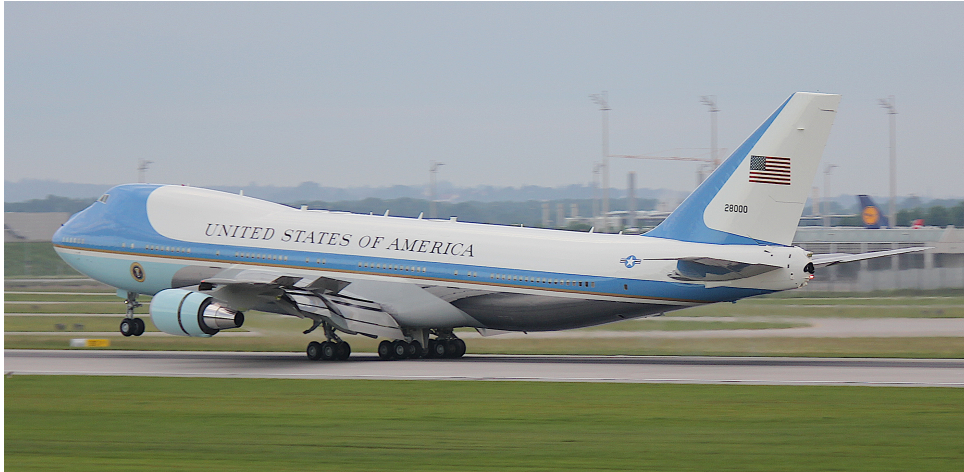
Figure 6.2: A Boeing VC-25A after touchdown on the runway. The deceleration devices are clearly visible.
