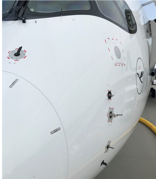
Figure 8.3: Air data sensors on the left side of the nose of the Airbus A350. The static port is located right below the windows surrounded by the red dashed line.
