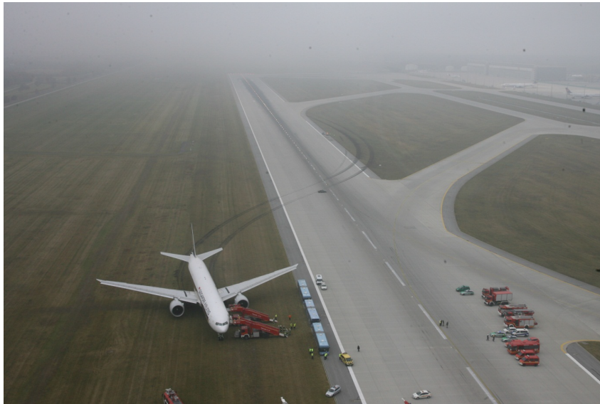
Figure 7.6: The RE (veer-off) accident at MUC/EDDM in 2011 [Bun11]. The tire markings are well visible.
