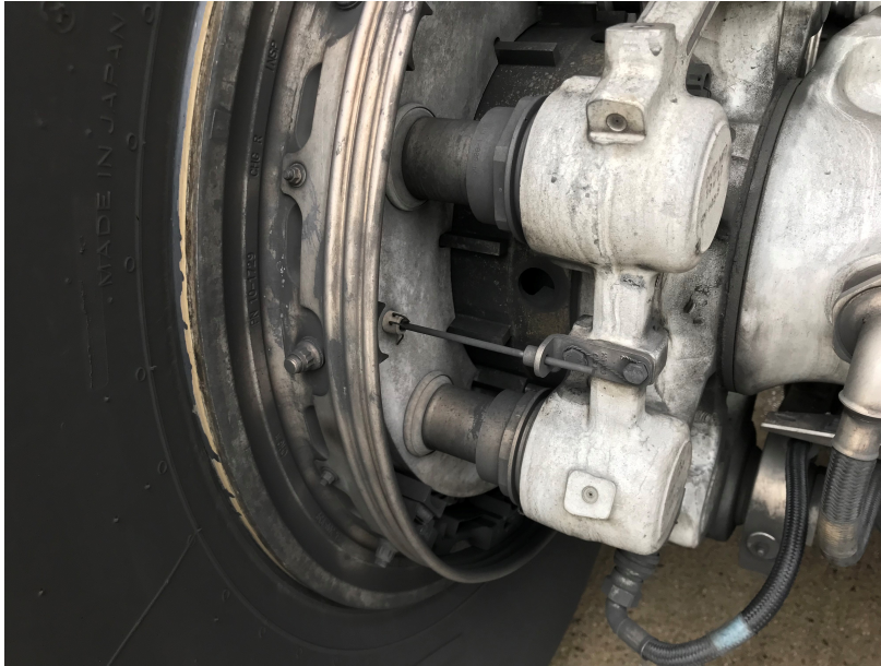
Figure 6.4: Braking disc on the main landing gear of a Boeing 777-300ER
