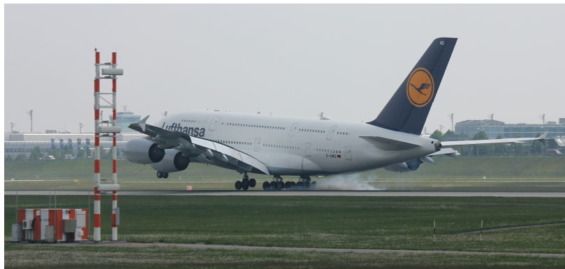
Figure 8.1: An Airbus A380 touching down on the runway with multiple landing gears. The glideslope antenna is visible on the left which is located abeam the desired touchdown point.
