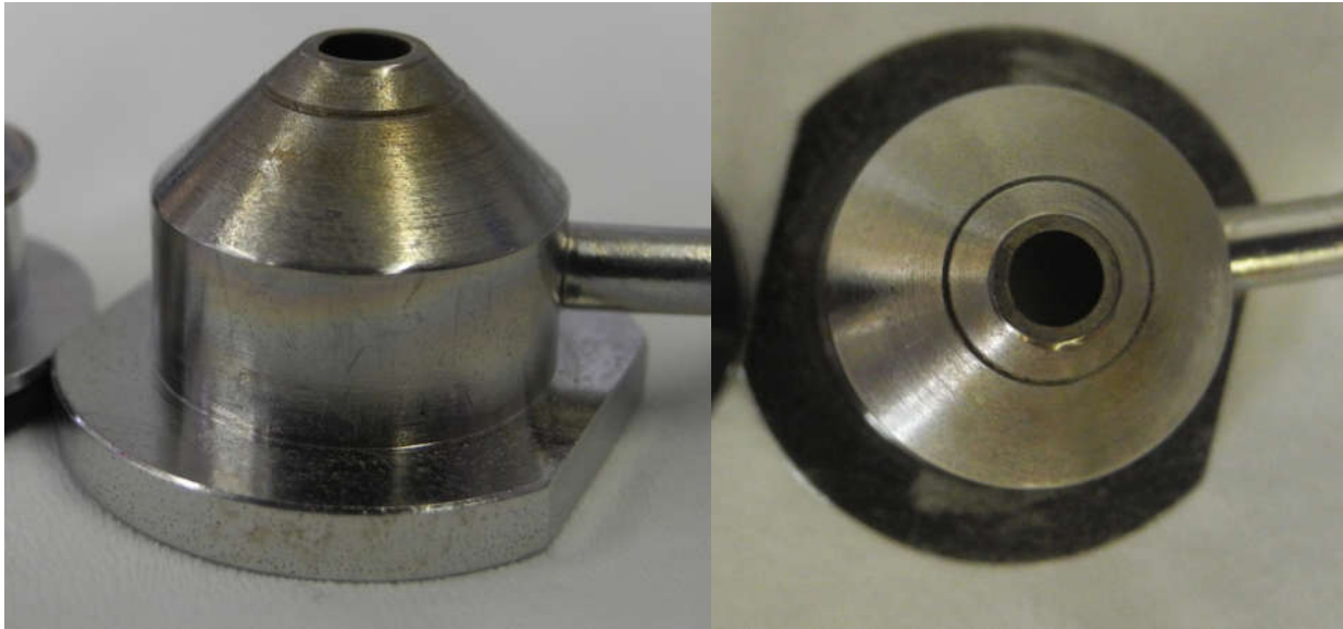
Figure 18: ESI spray shield after 40 analytical runs, including 10 waters blanks and 30 blood plasma samples, injections on Waters BEH HILIC column
