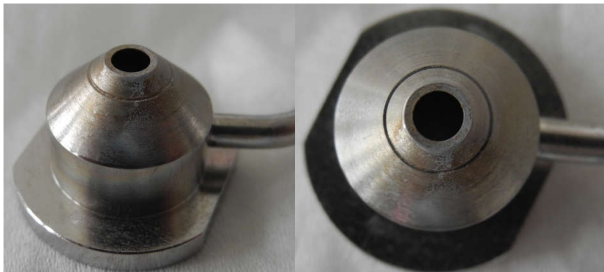
Figure 16: ESI spray shield after 40 analytical runs of blank (water) injections on Grace Vision HT HILIC column
