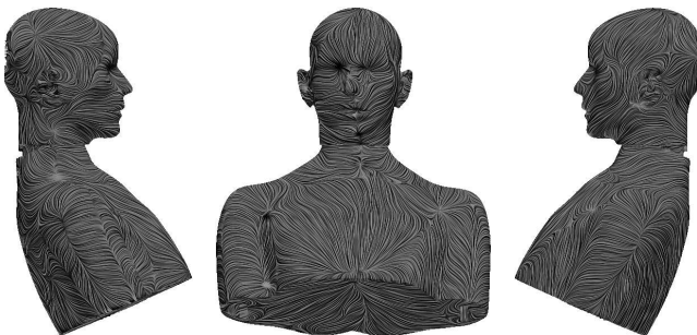
Figure 3.58: Line Integral Convolution (LIC) of the time averaged wall shear stress on the anthropomorphic dummy of the co-driver side. Left picture: view from side window, middle picture: front view, right picture: inner side view.
