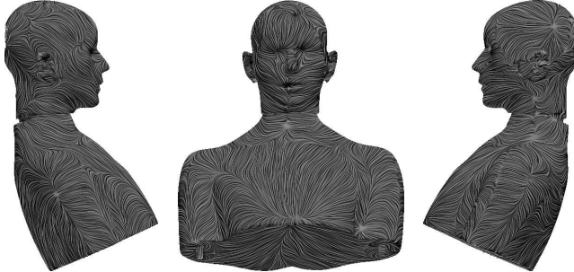
Figure 3.57: Line Integral Convolution (LIC) of the time averaged wall shear stress on the anthropomorphic dummy of the driver side. Left picture: inner side view, middle picture: front view, right picture: view from side window.
