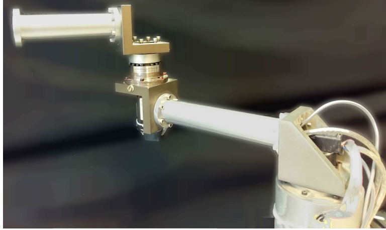
Figure 2.2: Two-DoF serial robot used in experiments.
