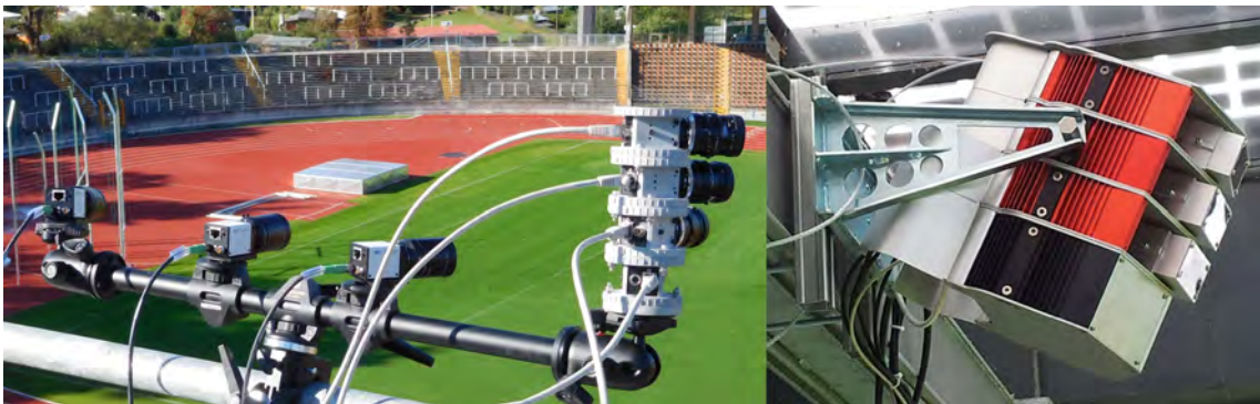
Figure 3.6: Three different examples of semiautomatic optical tracking systems. Left: STATS's SportVU and Pixellot camera system. Right: ChyronHego's Tracab Gen 4 system in a weatherproof casing.
