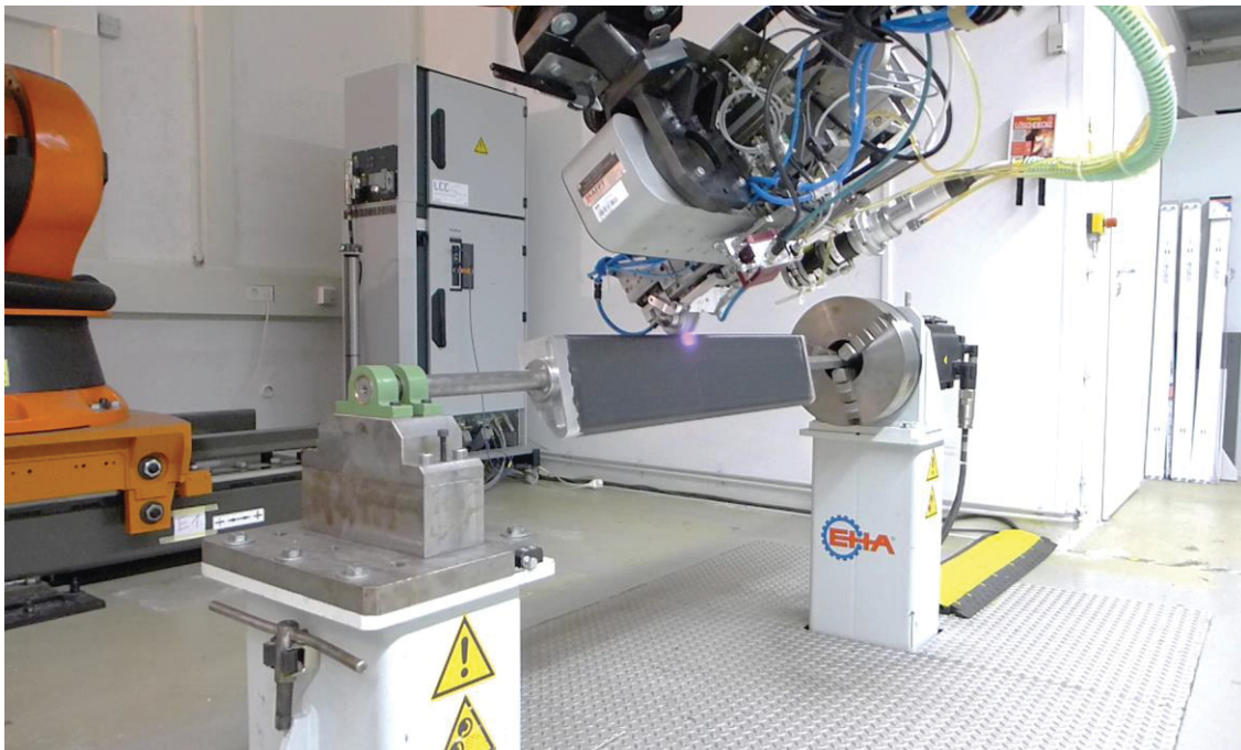
Fig. 7-15: Demonstrator manufacturing using a rotating axis
