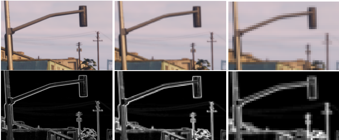
Figure 8.12: The images and the corresponding edge amplitudes of three levels in an image pyramid are displayed. From left to right, fine-scale structures are suppressed and edges may merge or disappear in the coarser pyramid levels.
