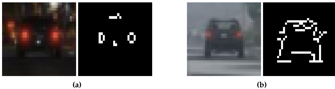
Figure 9.7: In (a), a model generated at night is displayed. The low contrast between the car and the road generates a model that is mainly focused on the lights of the car. These are not very descriptive and may easily be mistaken for any other car. In (b), a typical model that is generated in better lighting conditions is displayed..
