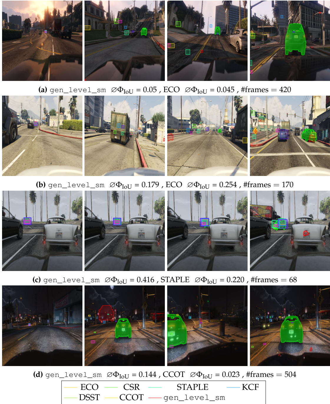
Figure 9.16: Challenging Sequences in which gen_level_sm and the other methods perform poorly are displayed. The \emptyset\Phi_{\text{IoU}} is displayed for the gen_level_sm and the best performing other method.
