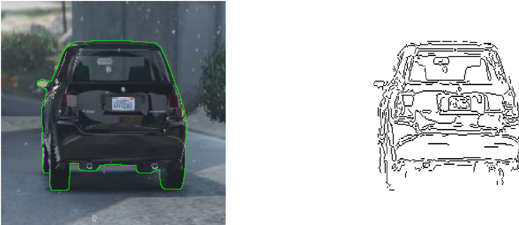
Figure 8.1: On the left, the typical input for the shape-based matching is displayed. The model initialization assumes the region (displayed as the green border) of the object is known. On the right, the points of the corresponding shape model are displayed.
