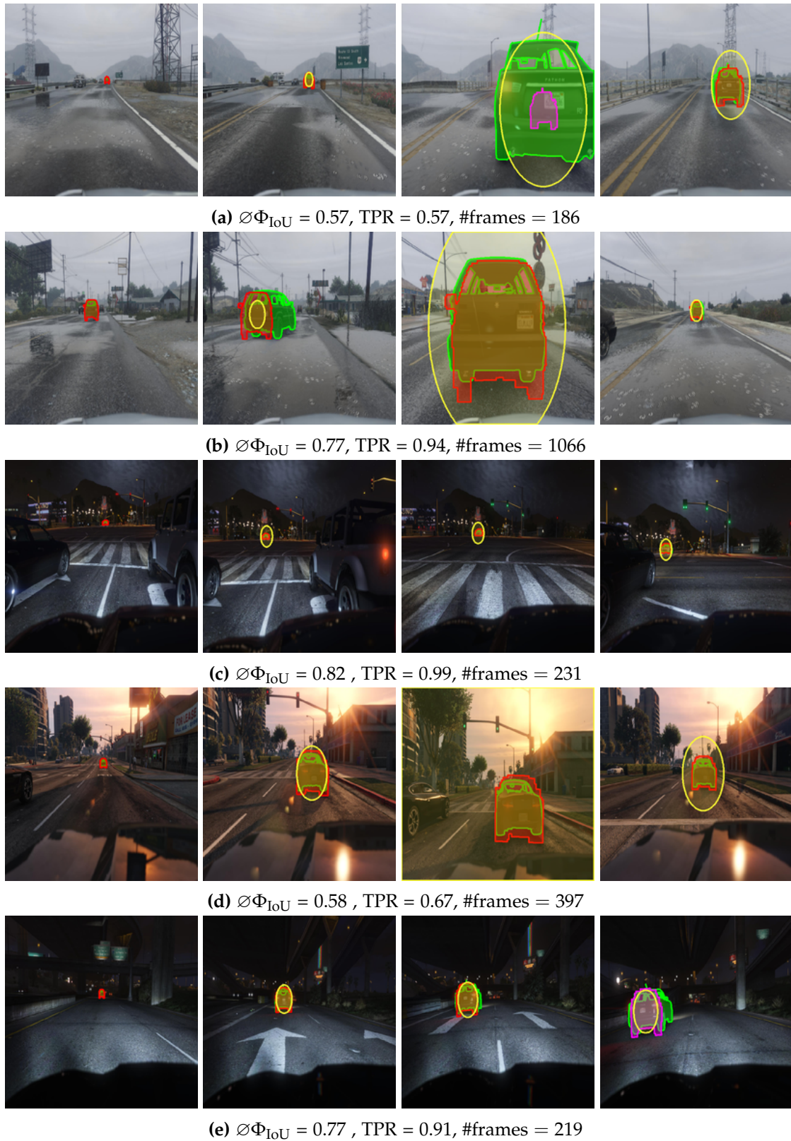
Figure 9.11: A collection of results from gen_level_sm . The tracker is able to track cars in various settings and in long-term sequences with more than 1000 frames (b).
