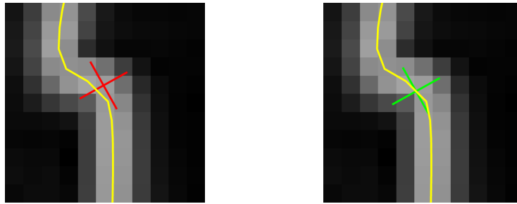
Figure 8.14: Scaling the model points to the coarser levels in the dynamic shape model pyramid generation may lead to model points (left image) that do not lie directly on the subpixel-precise image edges (yellow contour). In the right image, the respective model point that would be generated by the model initialization is displayed.
