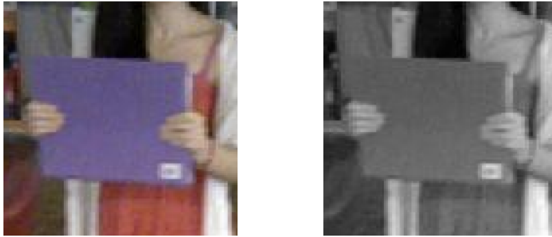
Figure 7.14: A close-up of book from VOT2016 [116]. The book is not an MSER in the gray-scale image since its background is lighter and darker than the book itself. Hence, it cannot be tracked with the existing MSER tracking. The book is a homogeneous region however, and can efficiently be tracked with the proposed MSHR tracking. See Fig. 7.13 for the overlap scores.
