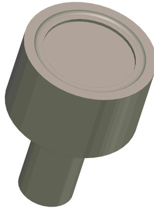
**Figure 6.4:** Schematic drawing of the manufactured upper part of the extrusion die fitting the exact dimensions of CR2032 coin cells. The metal die was lined with Teflon<sup>®</sup> to avoid short circuit.
