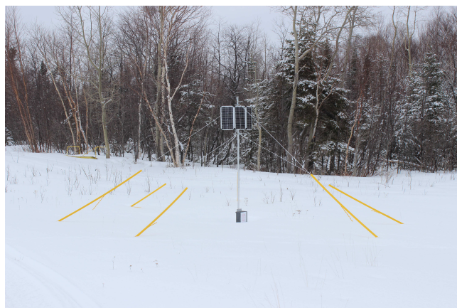
Figure 1. SnowSense station with solar power supply in Millertown in Newfoundland, Canada in April, 2018.
