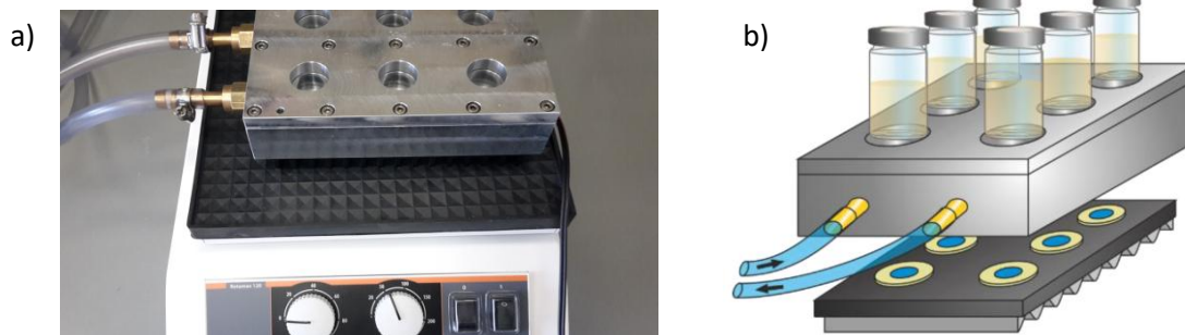
Figure S9. a) Image of the photocatalytic set-up combined with a horizontal shaker. b) Schematic image of the set-up including cooling block and LED array. [9]
