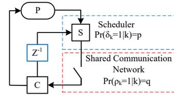
Fig. 2: A decoupled control loop of the shared contention-based communication network
