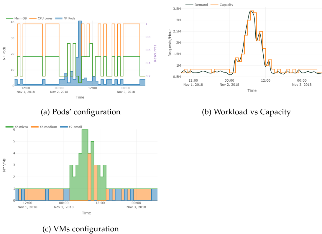
Figure 6.7: Scaling plan using Always Resize strategy
