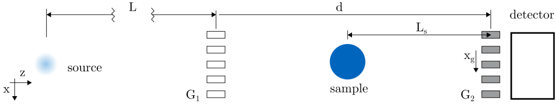
Figure 4.2: Schematic illustration of a Talbot interferometer. The phase-grating G_1 is positioned at distance L downstream of the source. An attenuation grating G_2 is placed at an appropriate distance d in front of the detector, given by Eq.(4.5). The sample is placed at a distance L_s upstream of the detector, here exemplary between G_1 and G_2 .
