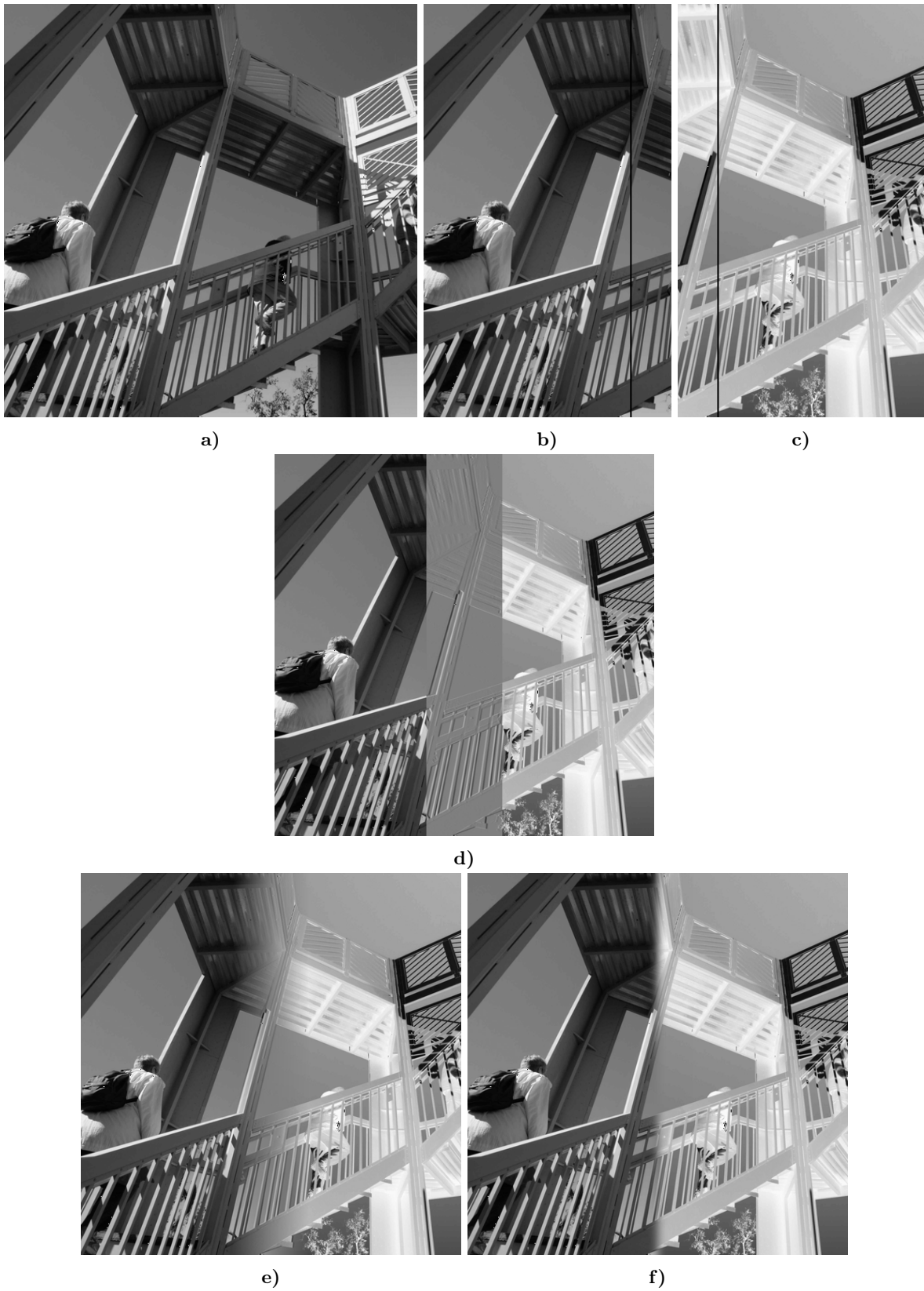
Figure 7.10: AN ILLUSTRATIVE EXAMPLE OF IMAGE STITCHING. THE ORIGINAL IMAGE, TAKEN FROM SCIPY.MISC.ASCENT , IS SHOWN IN A) [JONES ET AL., 2001]. B) AND C) SHOW OVERLAPPING REGIONS OF A), WHERE C) IS THE INVERSE OF THE ORIGINAL IMAGE, THE VERTICAL LINES INDICATE THE BORDER OF THE OVERLAP. D)-F) SHOW THE RESULT OF BLENDING THE IMAGES TOGETHER WITH A TWO-PIXEL MISMATCH AND DIFFERENT BLENDING FUNCTIONS. D) IS THE AVERAGE, E) IS A LINEAR AND F) A SIGMOID BLENDING.
