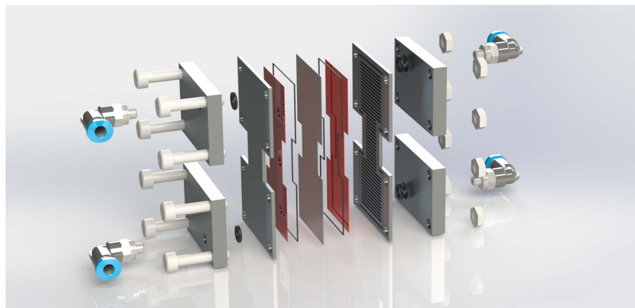
Figure 7.2: SCHEMATIC EXPLOSION DRAWING OF THE PROTOTYPE OF THE PEMFC USED IN THIS WORK. THE MEA IS SHOWN IN THE MIDDLE TOGETHER WITH THE GAS DIFFUSION LAYERS, CONTACTING PLATES WITH EMBEDDED FLOW-CHANNELS AS WELL AS THE OUTER ASSEMBLY FOR MOUNTING AND CONNECTION.
