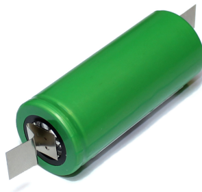
Figure 2.5: Photo of 26650-format cell Sony US26650FTC1. Reproduced from [18].
