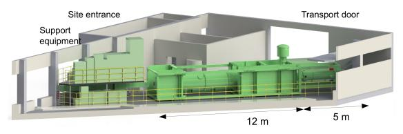
Fig. 9.10: PERC setup at the MEPHISTO beam facility in the Neutron Guide Hall East of the research reactor FRM-II.
