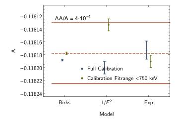
Fig. 7.13: Comparison of the combined result for the beta asymmetry A, when using different non-linearity models and fit ranges for the extraction of calibration parameters. The errorbars represent the projected calibration uncertainty of the given model. The region indicated by the red lines represents the estimate for the uncertainty. The results are also summarized in table 7.1.
