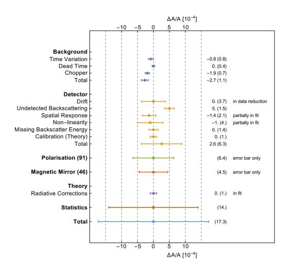
Fig. 9.1: Error Budget for the analysis of the beta asymmetry using a fit range of 297 - 604 keV. The corrections shown refer to the corrections necessary to correct the fit result obtained in section 6.2. The neutron beam polarisation and magnetic mirror effect corrections result from a seperate analysis and were blinded during the analysis. Both are shown only with the corresponding errorbars.
