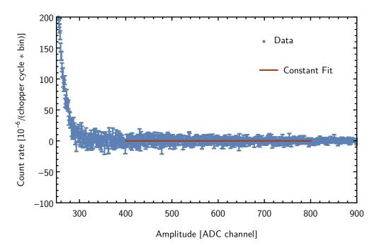
Fig. 8.9: Fit to the electron spectrum  $N^{\uparrow}(E_e) + N^{\downarrow}$  for detector 1 / 83 Hz above the electron endpoint energy. This fit is used to determine how well the background subtraction works. The results of these fits for all datasets are summarized in table 8.5.
