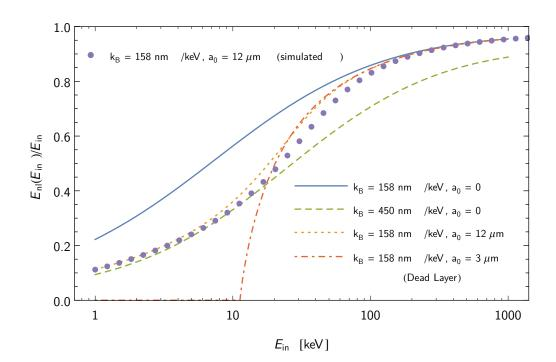
Fig. 7.5: Effective energy normalized to the incident electron energy for different strength of the Birks non-linearity with and without surface effects  $(a_0 \neq 0)$ .
