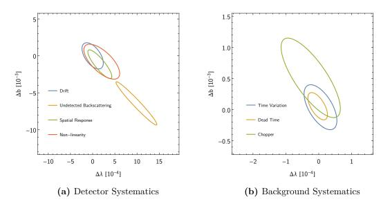
Fig. 9.5: Systematic effects related to background and the electron detector for the combined  $\lambda$ -b analysis. The corrections are represented by the centre of the ellipses, which denote the corresponding 68.27% C.L. uncertainty.
