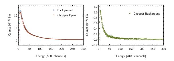
(a) Pulse height spectra extracted from the background time window and a time window that corresponds to the chopper being completely open (see equation 8.4.
