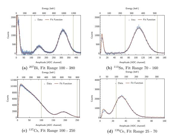
Fig. 6.1: Example for the measured calibration spectra and the simultaneous fit performed to extract the free parameters of the detector response model (see chapter 5).
