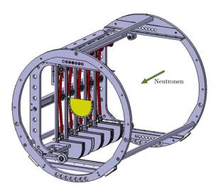
Fig. 3.7: Schematic of the scanner device used to move the five calibration sources inside the decay volume (from [Wil07].
