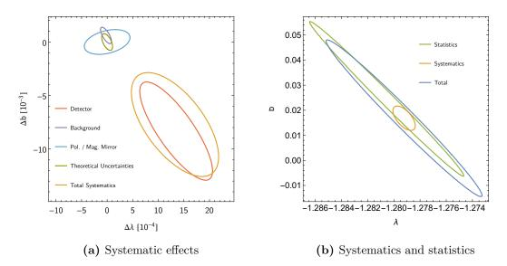
Fig. 9.6: Systematic effects related to background and the electron detector for the combined  $\lambda$ -b analysis. The corrections are represented by the centre of the ellipses, which denote the corresponding 68.27% C.L. uncertainty.
