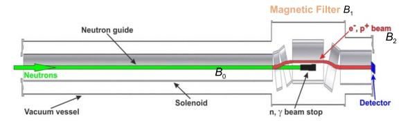
Fig. 9.9: Schematic of the PERC intrument.
