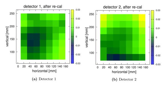
Fig. 6.3: Scan measurements performed during the 2009 beamtime taken from [Mes11]. The variation of the measured detector amplitude within the area covered the neutron beam is 1%.
