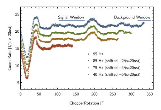
Fig. 8.4: Measurement of the chopper background using a NaI-counter for different chopper frequencies. The data show the reduction of background during the chopper opening at around 18 ° and a variation of the background while the chopper rotates. This variation induces differences of the background measured within the signal and background window. The intensity is normalized to the counts per second and time-of-flight bin with a bin width of 20  $\mu$ s.
