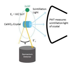
Fig. 7.2: Compton-coincidence setup to measure the intrinsic scintillator non-linearity as used in [Opp16]. The monoenergetic gammas emitted from the <sup>137</sup>Cs-source produce Compton electrons within the scintillator. The resulting scintillation light is measured with a photomultiplier in coincidence with the gamma that is detected by a Germanium detector. Image taken from [Opp16].
