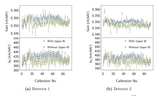
Fig. 7.11: Comparison of the detector calibration with and without the upper  $^{207}$ Bi-peak included in the fit using the Birks model with  $k_B$  free. Reducing the calibration fit range leads to less variations of the detector gain and non-linearity when comparing the individual results.
