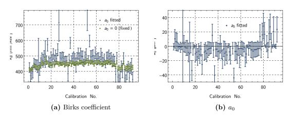
Fig. 7.6: Comparison of the resulting Birks coefficient  $k_B$  with and without considering surface effects within the fit and the resulting thickness parameter  $a_0$ .
