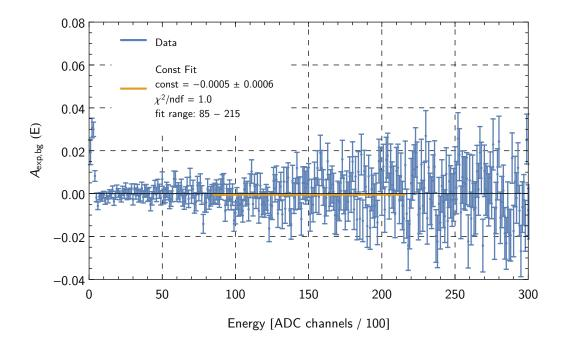
Fig. 8.10: Constant fit to the background asymmetry spectrum of one of four datasets according to equation 8.20. The results are limits by the number of background events and show no spin-dependence of the background.
