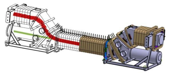
Fig. 3.4: The spectrometer PERKEO III. The image shows the coil system (brown) and vaccum vessel (blue). On the left side of the picture the neutron beam is shown as green line and the electron trajectories are indicated as red lines.
