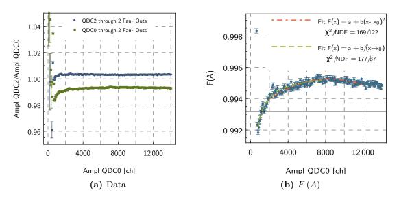
Fig. 7.9: Comparison of the measured amplitudes when guiding PMT pulses through a single or two fan-outs. Calculating F(A) according to equation 7.22 shows that the damping in the second fan-out stage is amplitude dependent.
