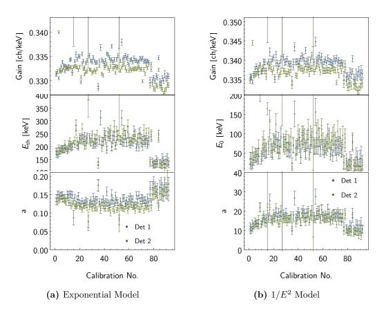
Fig. 7.10: Results for the individual calibration parameters when extending the scintillator non-linearity (with  $k_B = 150 \text{ nm/keV}$ ) with an Exponential or  $1/E^2$  model. The errorbars denote the correlated uncertainties for the parameters.
