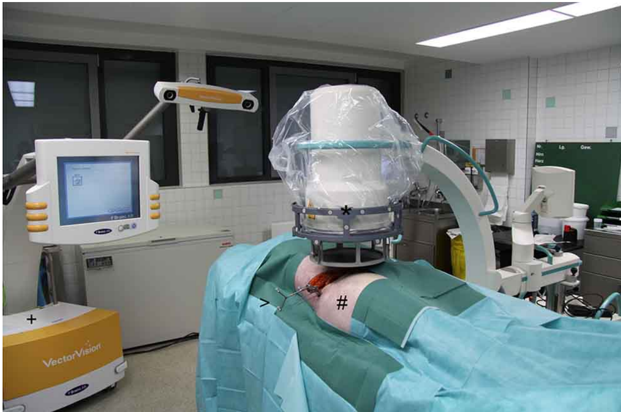
Figure 14 – First position of C-arm during registration
