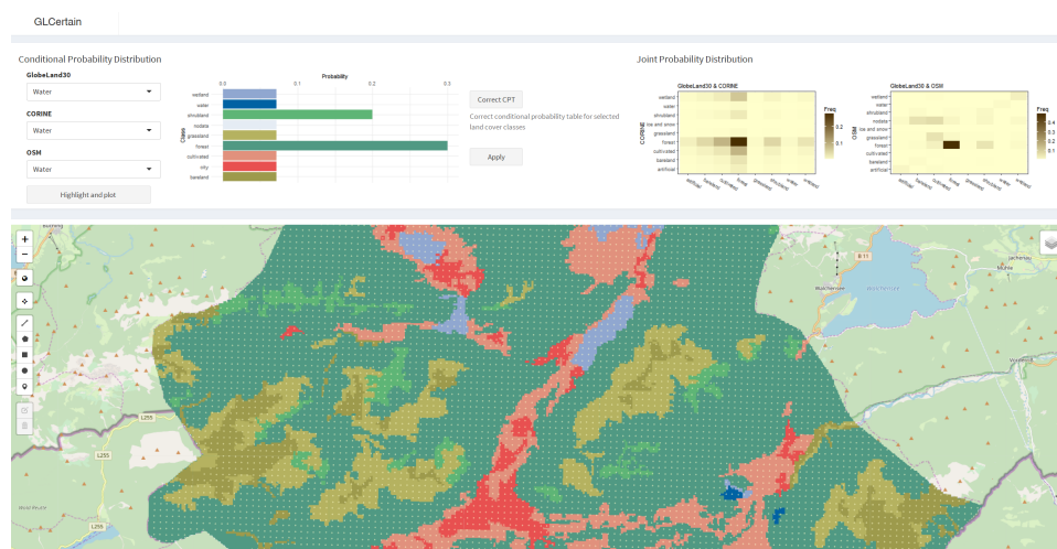
Figure 5.8: Uncertainty-Aware visual analytics interface. The graphical UI includes Conditional Probability Panel, Joint Probability Distribution plots, and Map panel.
