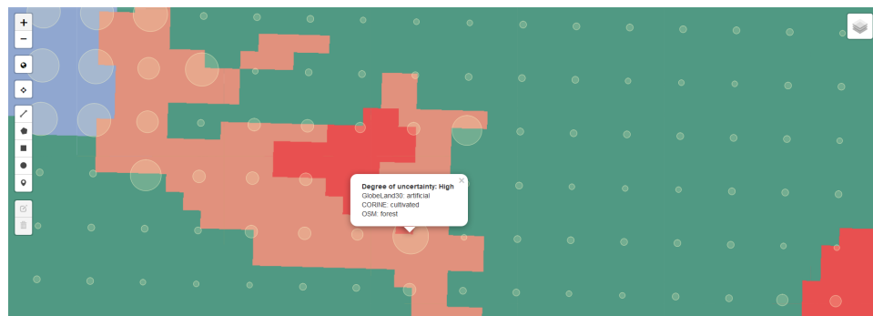
Figure 5.11: Map view illustrates the categorical maps of land cover and with an overlay of proportional circles that identify the amount of entropy measured as the Shannon Index. The larger the entropy, the larger the circle symbol will be.
